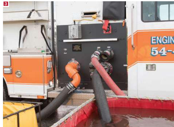
2 Engine 54-4's pump panel is laid out for ease of operation, including the suction inlet control valves and their corresponding air primer controls. 3 Engine 54-4's dual suction inlets on the officer's side.
