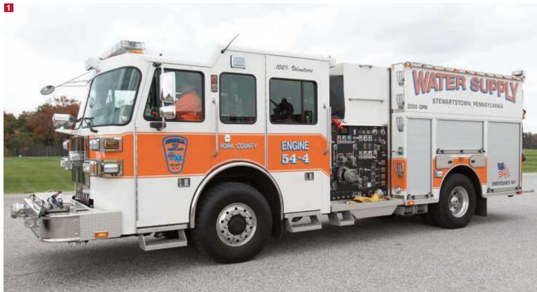
1 Engine 54-4 from the Eureka Volunteer Fire Department, in Stewartstown, Pennsylvania, is a 2015 Sutphen pumper equipped with a 2,250-gpm Hale XS pump. (Photos by author.)
